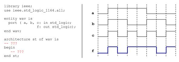
d) Complete the timing diagram of the following circuit: (6 pts)
