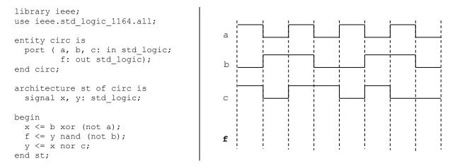
c) The following is the timing diagram of a logic circuit with 3 inputs. Sketch the logic circuit that generates this waveform. Then, complete the VHDL code. (8 pts)
